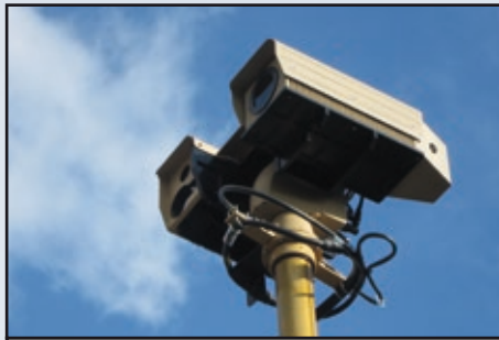
Piranha LRTV camera option, mast mounted on a vehicle
