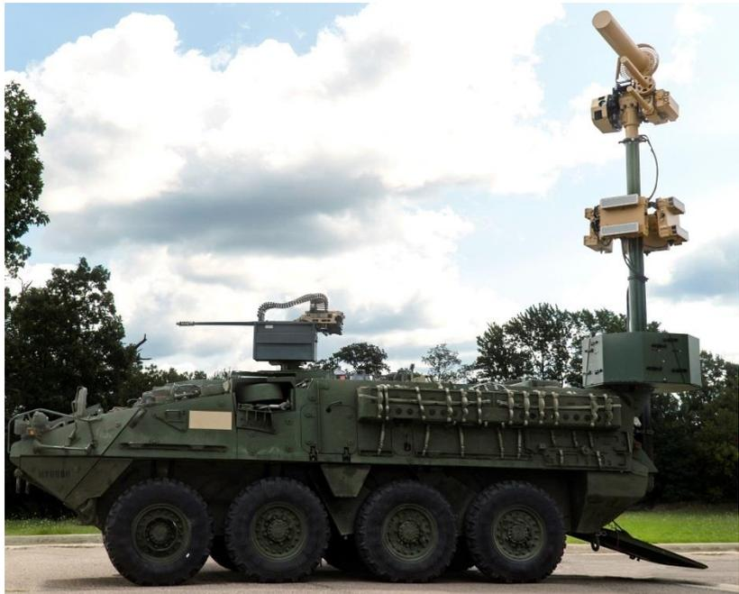
Orbital ATK's T-REX concept comprises the integration of the Liteye mast-mounted C-UAS solution on board a Stryker vehicle with networked M230LF 30mm cannon.
